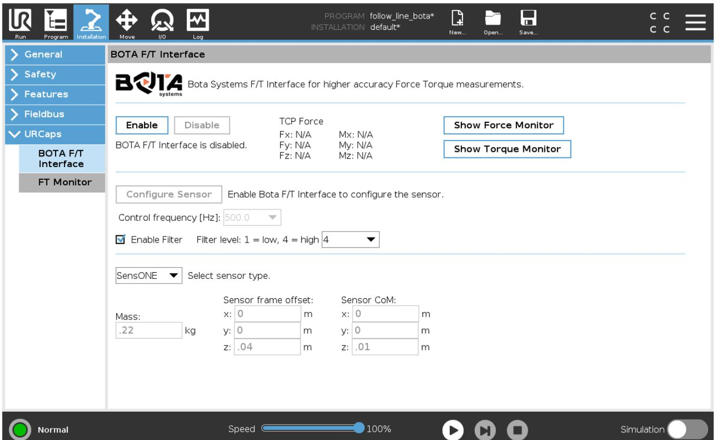
To ease the setup of your application, there is the option to plot the forces and torques. Tap either on **Show Force Monitor** or **Show Torque Monitor** to open a window that shows the current force or torque stream (containing the last 1200 measurements). Tap on Close to close the window again and return to the installation menu. Note that you can see the current TCP force after enabling the sensor. However, only after starting a program it will use the external F/T sensor.
